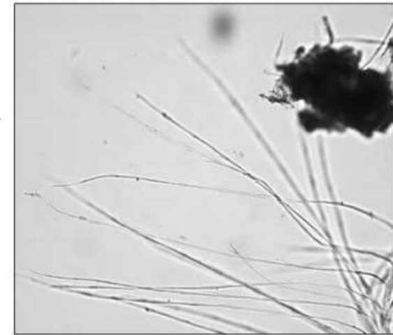
Figure 3. Photomicrograph of a downy feather sample collected from the tail section of the Cessna Citation that crashed near Wiley Post Airport, Oklahoma. The diagnostic microscopic characters of the downy barbs in this sample include short barbules with long, distal prongs.
